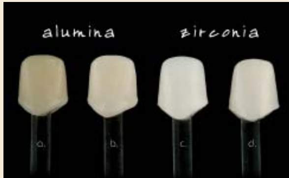
Fig 41 The influence of fluorescent stains on the value and chroma of alumina and zirconia copings under natural light: (a and c) without fluorescence; (b and d) with fluorescence.
